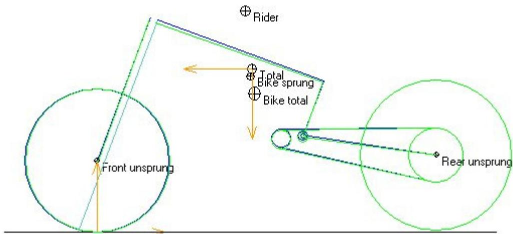
Above braking position is shown with different front fork oil levels. Rear wheel is lifted from the ground.
