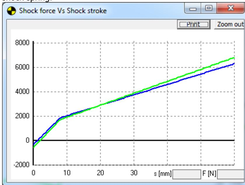
When you want to keep same bike position in mid corner, find your shock stroke @ mid corner position from data. Make 2 setups in SuspAct: 1 with standard spring and preload and 1 with modified spring and changed preload.
