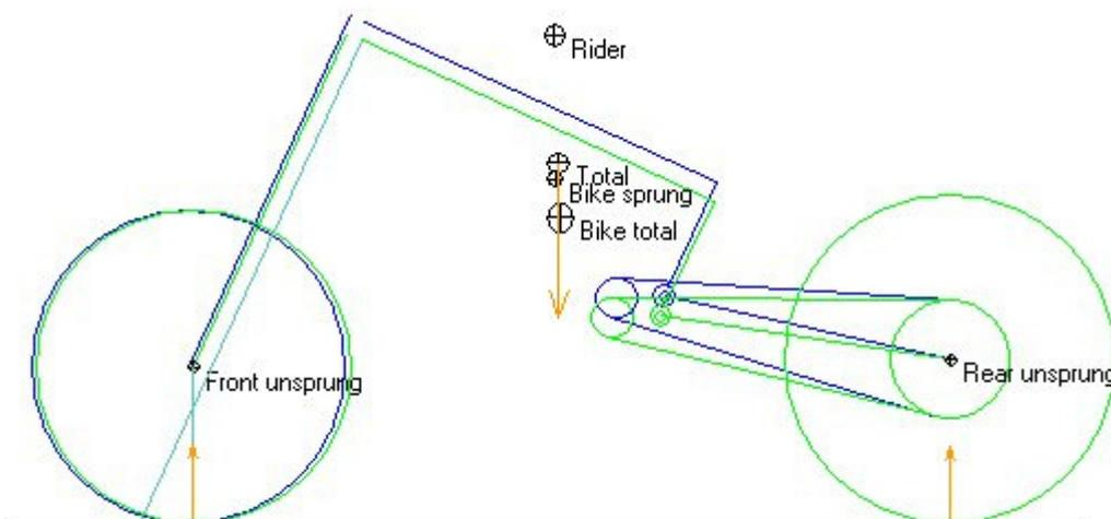
The arrows in orange display the force vectors. In this picture there is a vertical load from the total bike + rider CoG, which is supported by two vertical tire forces.
