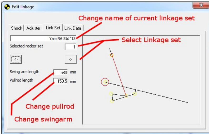
Depending on the bike model there might be different link sets defined in your bike model. This is normally the case for SBK or GP racing bikes where the linkage can be changed according to the rules for that class. Most production bikes will have 1 linkage defined.
