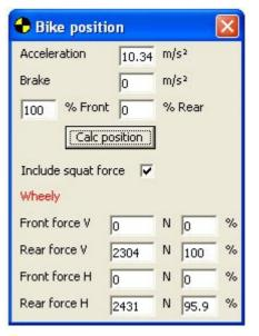
The example bike has a maximum acceleration of 10.34  $m/s^2$ , which is limited by wheely as can be seen by the red text.
